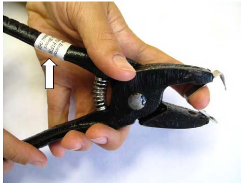
Figure 6: Loading a flipper tag into tag applicator. The arrow indicates which handle should be up.
