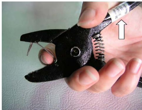
Figure 7: A fully seated tag in the tag applicator pliers.
