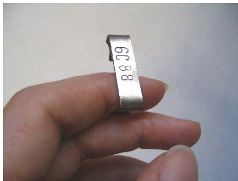
Figure 5: Holding a flipper tag in correct orientation to load into applicator. Note that the number side of the tag is up.
